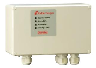
The FCS-LWM-1 is a Linear Heat Detector for detecting fire. Its functionality is based on the change in resistance of an electrical conductor caused by a rise in temperature.
