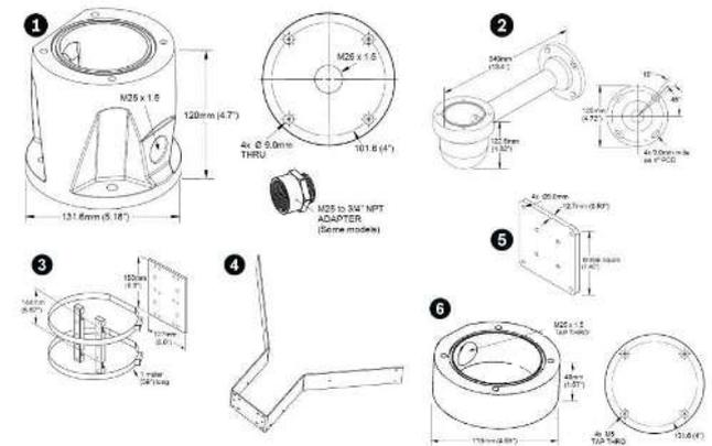
Fig. 1: Optional Mounts, MIC IP 7100i series
